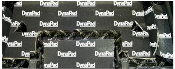
**The Hoodliner®** is made from 3/4" acoustic sound soaker foam with a reinforced, reflective mylar skin. The mylar skin is cleanable, oil and water resistant and provides 97% heat reflection. The Hoodliner has a high-tack pressure sensitive adhesive for easy peel and stick application. Great for engine or generator compartments.
